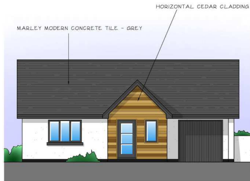
NORTH WEST ELEVATION
