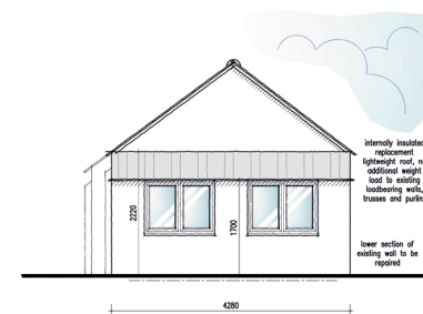
Proposed Side Elevation Scale 1:50
